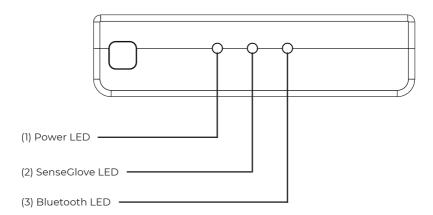
The power LED turns on as soon the device is powered. The color will indicate the battery level. Green > 40%, Orange 15% - 40%, Red < 15%.
